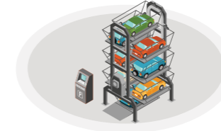
SEPARATE PARKING ELEVATORS
